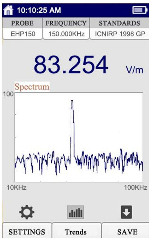
Spectrum mode is new added in the isotropic electric and magnetic field as one probe, which can be used to ascertain the main pollution sources in the environment quickly.
